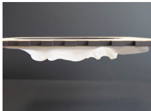
Figure 11, 12, 13, 14: 3D printing on textiles
